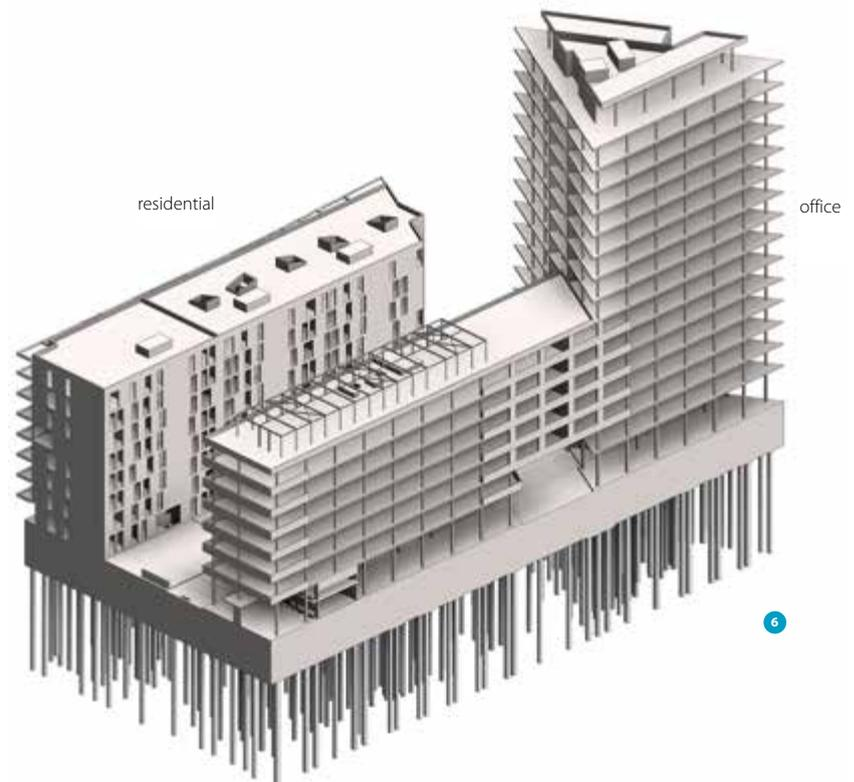
All plans produced by Schüßler-Plan are shown in a continuous, spatial 3D model in order to optimise the support structure, details and planning (fig. 6).
