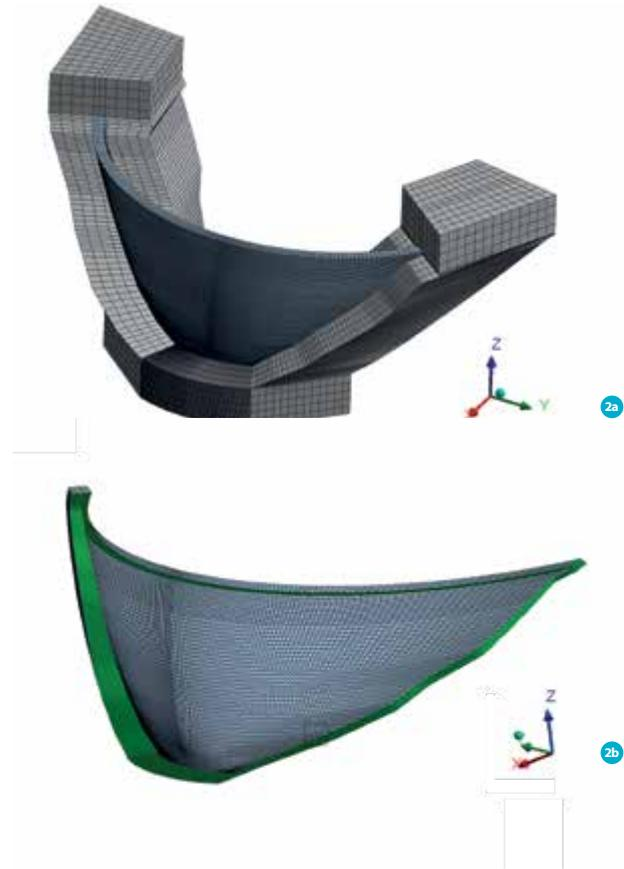
the design of the dam. If the dam was modelled fixed to the bedrock, this would lead to very high reinforcement intensities in the vertical direction in the lower part of the dam on the water side due to clamping of the three-dimensional shell structure. This was found unfeasible since it would require a large amount of anchors/bolts and consequently it would increase the construction cost substantially. Modelling the dam
