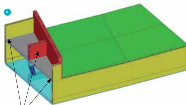
The 800 mm wall is equipped with three buttresses, which according to the console principle, partly absorbed collision loads during construction when a speed limit for passing vessels is applicable. After construction phase, these collision loads from vessels passing at normal speed are taken by the entire ridge structure.
