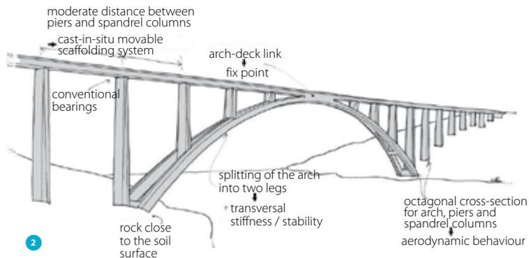
cable-stays from two temporary steel towers, using form travelers specially designed for this bridge; while the deck was constructed using an overhead movable scaffolding system (commonly used method in Spain for HSR concrete box-girder viaducts).
