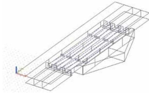
anchored to the existing girder webs (photo 9). Beside resisting loads during transient situation (prior to application of post-tensioning), this longitudinal reinforcement will also be active in persistent situation, together with the longitudinal post-tensioning.
