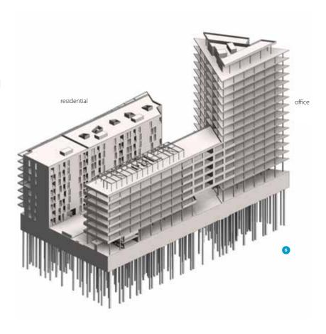
All plans produced by Schüßler-Plan are shown in a continuous, spatial 3D model in order to optimise the support structure, details and planning (fig. 6).
