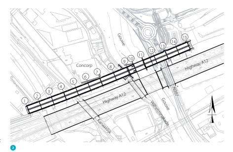
eastern approach ramp (124 m), the bascule pit and steel leaf (together 45.5 m) and the western approach ramp (280 m, all lengths approximate). The required  $2 \times 2$  lanes, in combination with a median of about 3 m width (ensuing from the landscape plan), and bevelled fibre reinforced plastic edge elements (ensuing from the visual quality plan) result in a total deck structure width of approximately 21.6 m (fig. 4).
